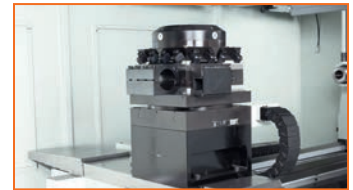
4-pos. hydraulic tool changer
