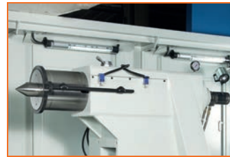
Tailstock with hydraulic quill
