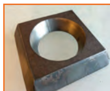
Bevel in 12 mm (0.47") St37 steel
