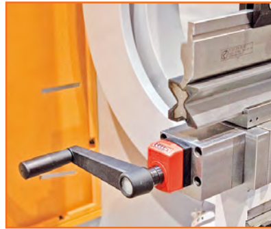
Optional Manual Crowning System (above) and CNC Motorized Crowning System (left)
