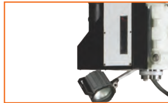
Z axis quill drive with ballscrew (CNC)
