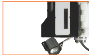
Z axis quill drive with ballscrew (CNC)
